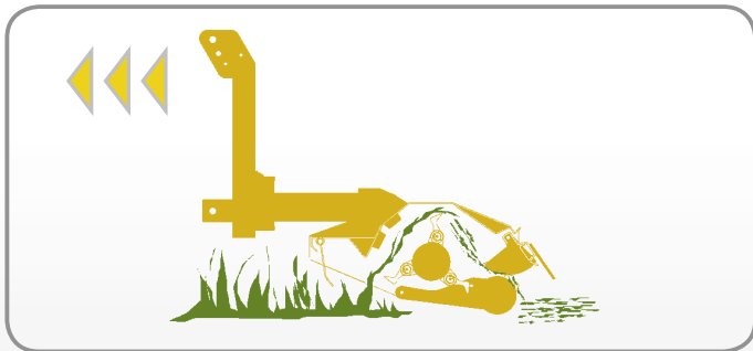
Open rear hood: to mulch grass with low power consumption
